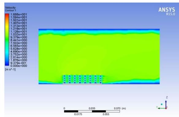
Fig:7 velocity contour on HEAT SINK of hollow fins with Rectangular perforation
