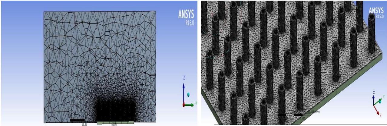
Fig: 3 Meshing of fins inside the enclosure
