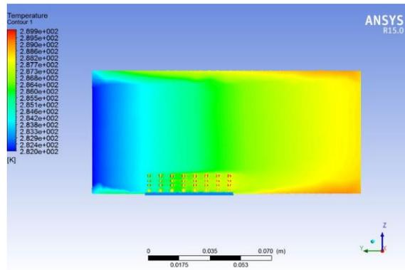
Fig:5 Temperature contour on HEAT SINK of hollow fins with Oval perforation
