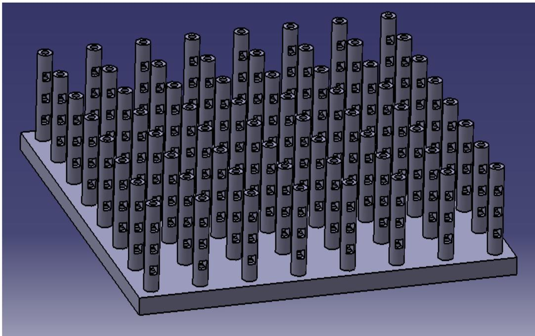
Fig: 1 Heat sink Model with hollow fins and Rectangular perforation.
