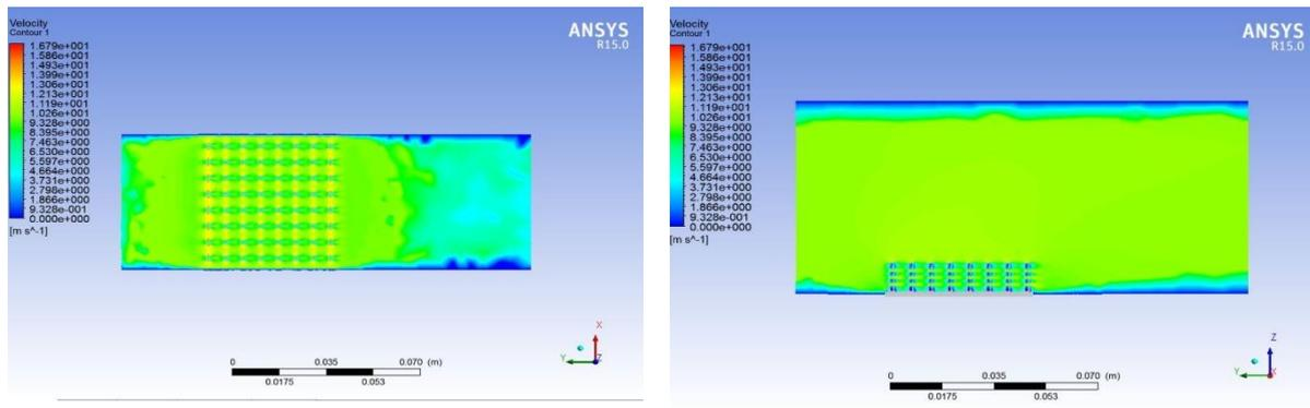
Fig:8 velocity contour on HEAT SINK of hollow fins with Rectangular perforation
