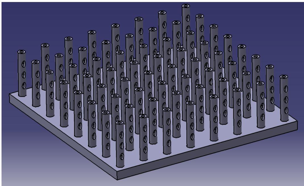
Fig: 2 Heat sink Model with hollow fins and Oval perforation.
