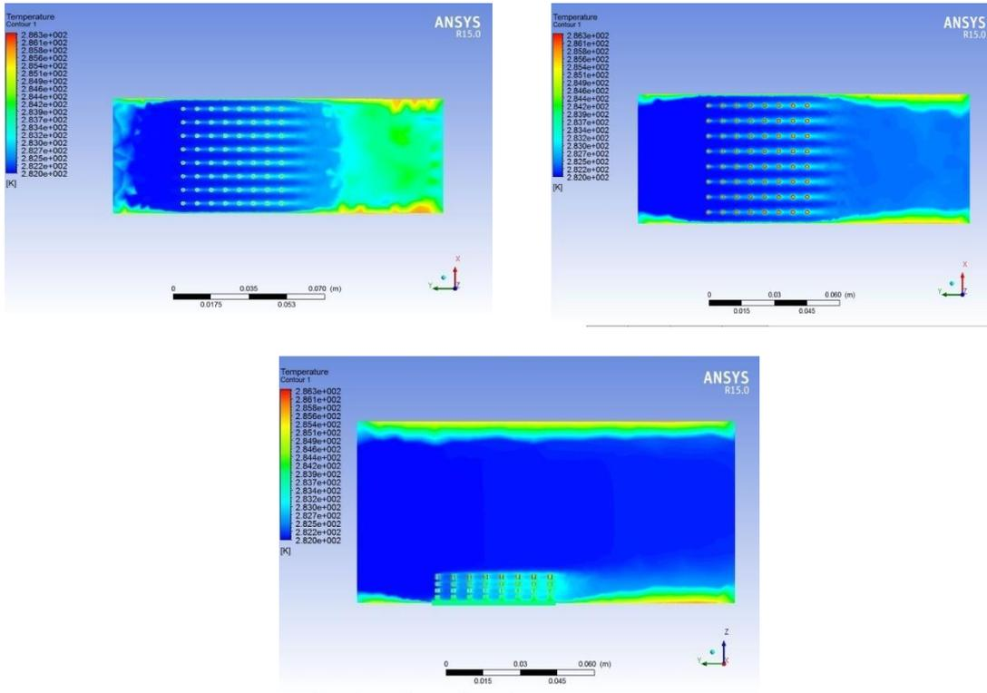
Fig:4 Temperature contour on HEAT SINK of hollow fins with Rectangular perforation
