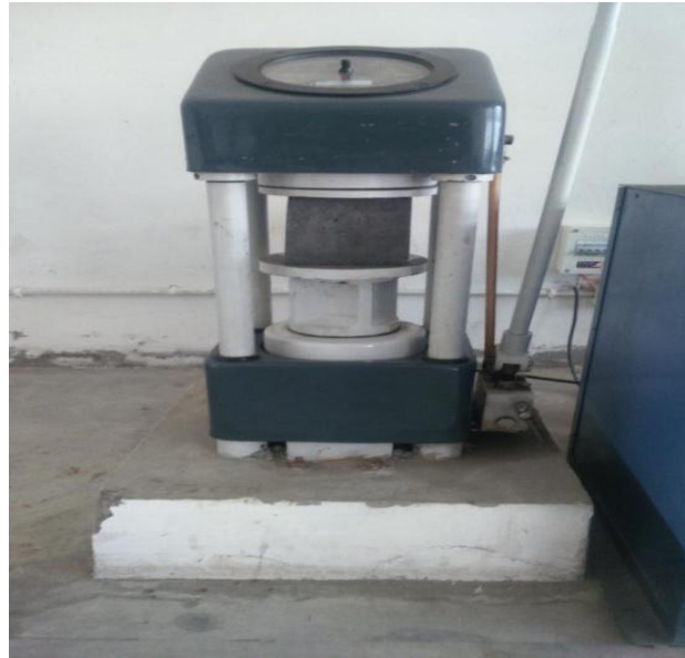
Fig 1: Compressive Strength testing Machine
