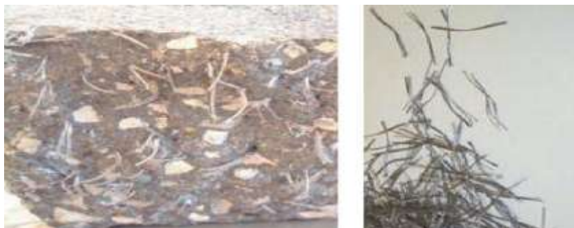
Fig.2. Polypropylene fibers give protection against Spalling [12].
