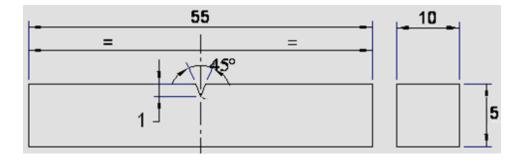
Dimension view of the impact testing specimen.
