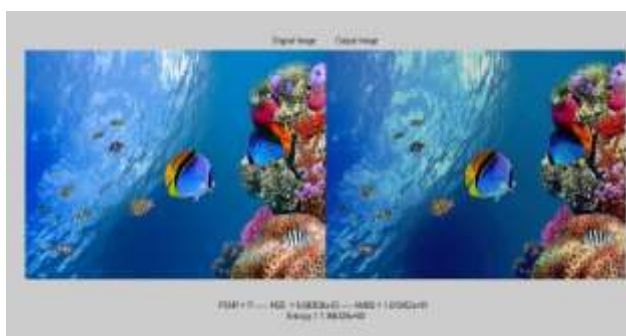
Fig.3 : Image of blue sea. Left image is original image and right image processed using Recursively Separated and Weighted Histogram Equalization Method
