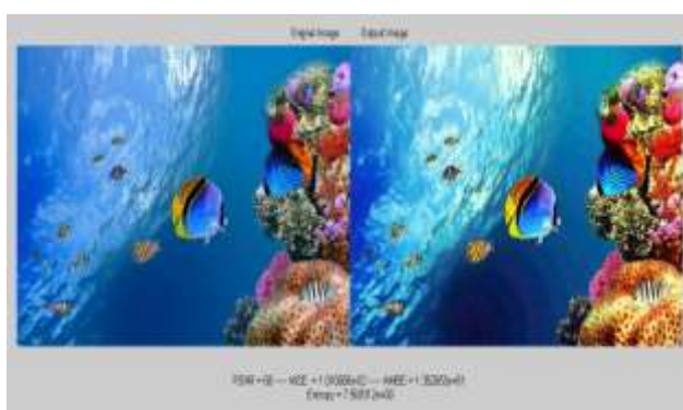
Fig.2 : Image of blue sea. Left image is original image and right image processed using Brightness Preserving Bi-Histogram Equalization Method
