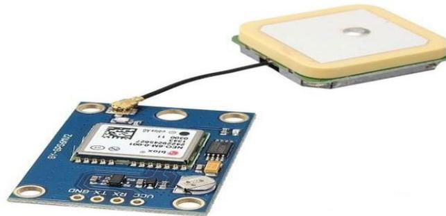
Figure 2. GPS Module (NEO-6M)
