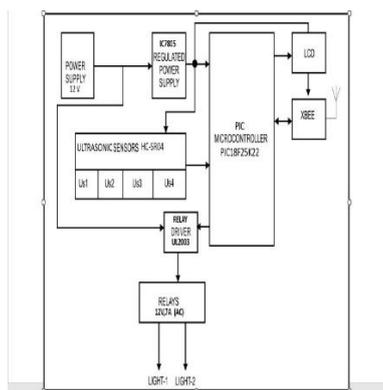
Fig (a): Block Diagram
