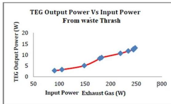
TEG Output Power Vs Input Power The graph shows that at the engine speed of 3736 rpm, input power of exhaust gas is 248.03 W & the TEG output power is 10 W, hence the overall efficiency obtained is 5.28%.
