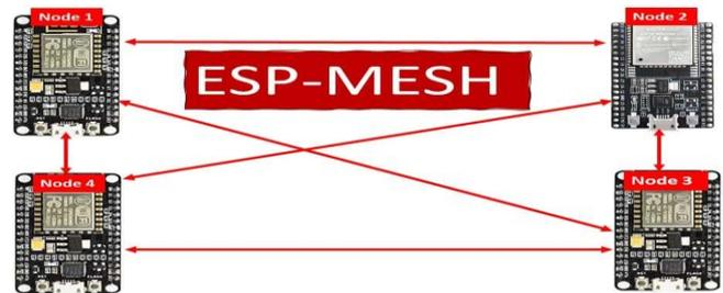
Fig 5a. ESP32 acting as Logger and providing a Mesh Topology
