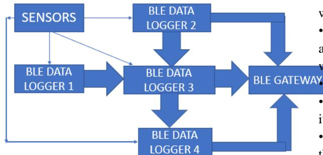
Fig 3. Block diagram of Development of Bluetooth Low Energy based Mesh Network Logger.
