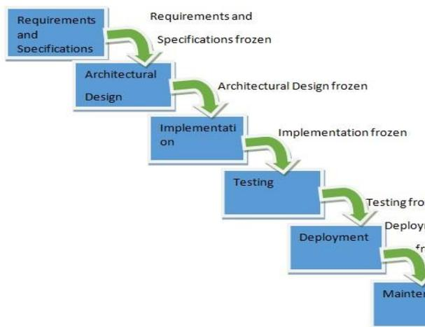
Figure <a>: The sequential phases in Waterfall model
