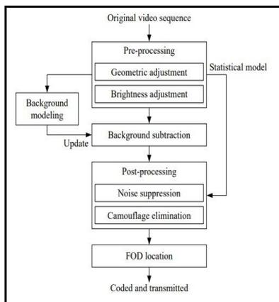
Fig. 4. Flowchart of FOD Detection System
