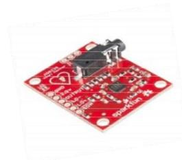
Fig.6. ECG Sensor
