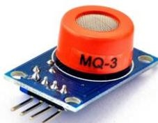
Fig 6. MQ3 Sensor Module
