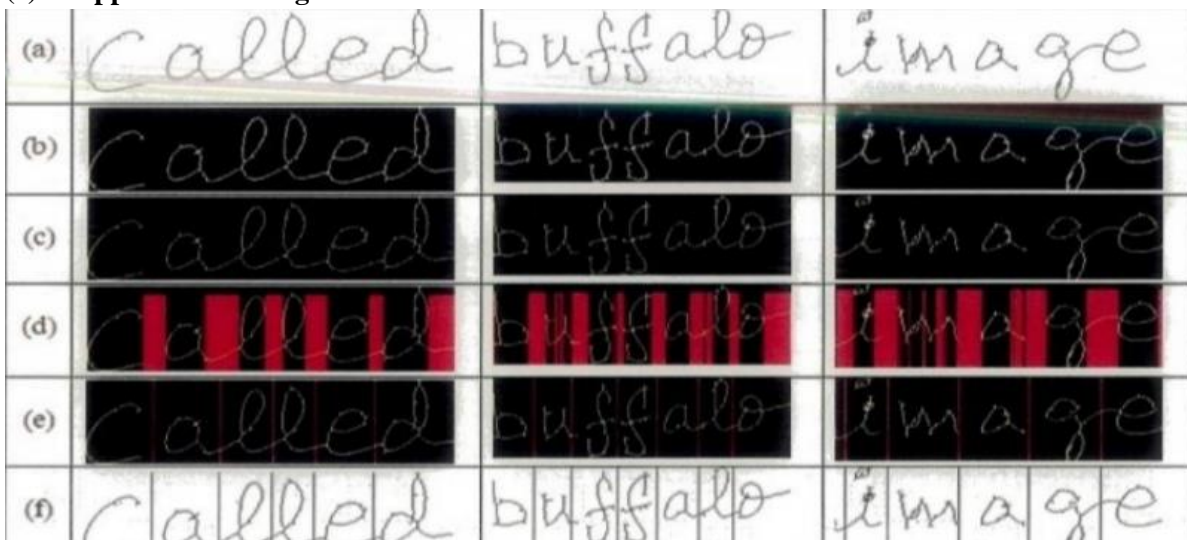
Fig. 1.10 Word Images Segmentation (a) Pre-processed word Images; (b) Inverted Binary Images; (c) RGB images; (d) Over-Segmentation in Images; (e) Image after removing Over-Segmentation; (f) Final Segmented Output Word Images
