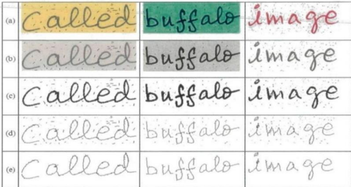
Fig. 1.9 Word Image preprocessing (a) Input Scanned Word Images; (b) Word Images after Gray Scale Intensity Threshold; (c) word Images in Binary Format; (d) Word images after thinning ; (e) Cropped Word Images after Noise Removal
