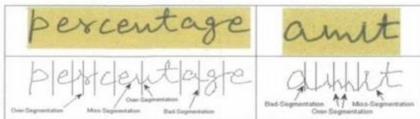
Fig. 1.11 Word Images showing All Type of Segmentation Errors
