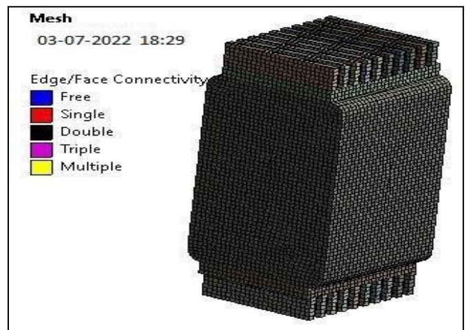
Figure: Meshing of Air Cooling Model (Isometric View)
