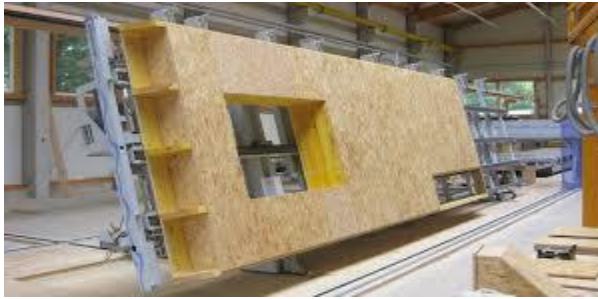
Fig 3.2 Prefabrication In Housing Construction
