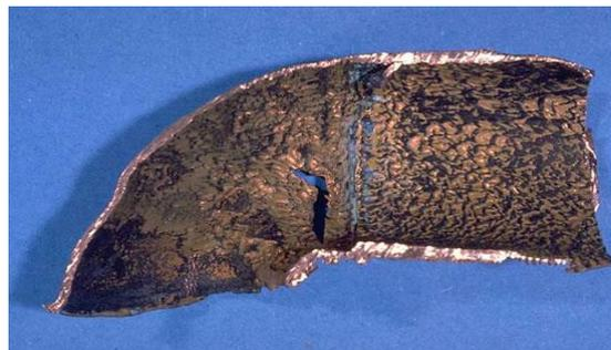
Figure 1: Erosion and Corrosion damage in pipe elbow
