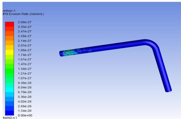
Figure 5: Erosion while diesel as a fluid medium
