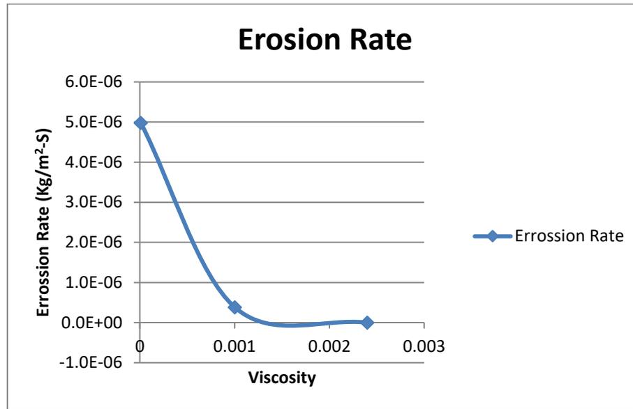
Figure 8: Graph between erosion rates VS Viscosity
