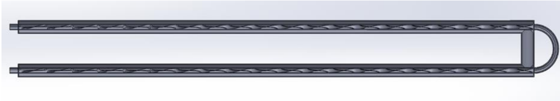
Figure 3: design 1 with aluminum strip inside inner tube
