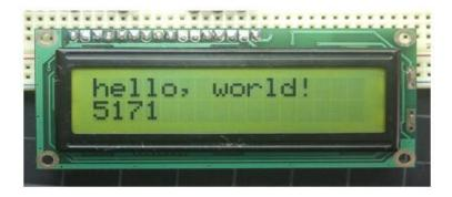
The LCDs have a lateral interface, bearing that the microcontroller has to preside several interface pins at once to control the display. The interface consists of the following pins:
