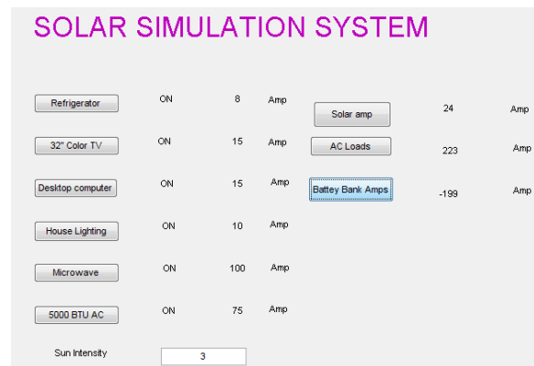
FIGURE 5 REFRIGERATOR, TV, DESK COMPUTER, HOUSE LIGHTING, MICROWAVE, 5000 BTU AC IS ON & SUN INTENSITY IS 3.SOLAR PANEL AMPS, BATTERY BANK AMPS WHEN REFRIGERATOR IS ON.
