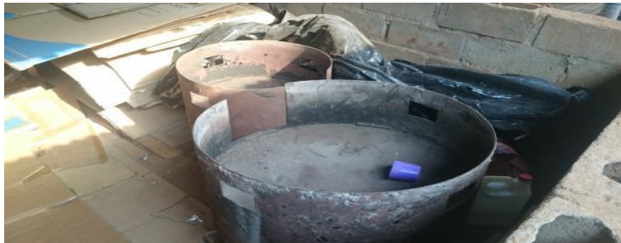
Fig.2 Vat for Heating & Mixing of Plastic Waste
